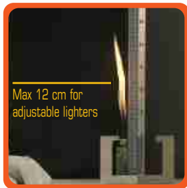
Failure to comply with the ISO 9994 Flame Height Test
