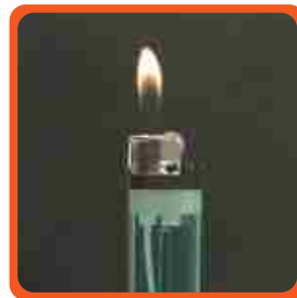
Failure to comply with the ISO 9994 Flame Extinction Test
